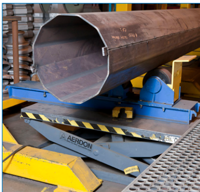
Use height-adjustable rollers or work tables to position work between your waist and your shoulders, close to your body.
