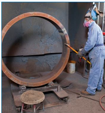
Use specialized rollers to position work between your waist and your shoulders, close to your body.
